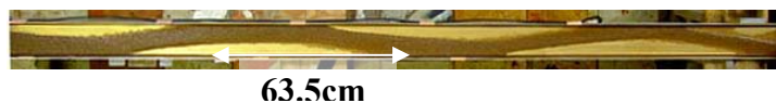
Figure 4. Medium sand ( d_s = 600-850 \mu\text{m} ); Fully developed meander structure, m_t = 10.2 \text{ g min}^{-1} , Fr_1 = 1.45 (data label E in Figure 1)
